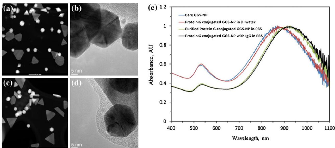
FIGURE 3. STEM (a, c) and high resolution TEM (b, d) images of the bare GGS-NPs and ProG-conjugated GGS-NPs: (a) and (b) Bare GGS-NPs. (c) and (d) Purified ProG-conjugated GGS-NPs. The NIR spectra of the bare and bioconjugated GGS-NPs (e).
