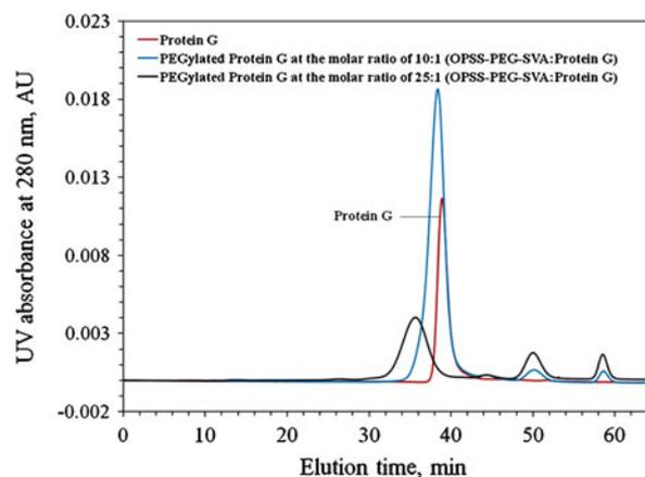
**FIGURE 2.** SEC-HPLC chromatograms of the PEGylated ProG with OPSS-PEG-SVA at two different molar ratios of OPSS-PEG-SVA to ProG: 10:1 and 25:1. ProG was used for comparison with PEGylated ProG. The elution buffer was pH 7.4 PBS consisting of 5 mM phosphates, 10 mM KCl and 140 mM NaCl. The elution flow rate was 0.3 mL min<sup>-1</sup>.
