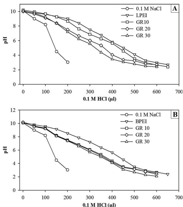
**FIGURE 6.** Titration curves of (A) LPEI and PEG-g-LPEI and (B) BPEI and PEG-g-BPEI. The slopes of the titration curves for linear PEI (A) between pH 7.5 and 4.5 are LPEI =  $-0.017$ , GR10 =  $-0.016$ , GR20 =  $-0.016$ , and GR30 =  $-0.018$ . The slopes of the titration curves for branched PEI (B) between pH 7.5 and 4.5 are BPEI =  $-0.017$ , GR10 =  $-0.015$ , GR20 =  $-0.016$ , and GR30 =  $-0.016$ .
